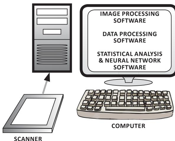
**Figure 4.** Schematic diagram of the computer vision system using a flatbed scanner as image acquisition device and a computer to process the image.
