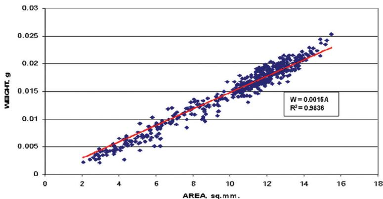
**Figure 13.** Comparison of predicted and actual weight of milled rice grains based on projected area
