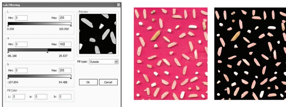
**Figure 9.** The GUI for background segmentation (a) and the milled rice image before and after background segmentation (b)
