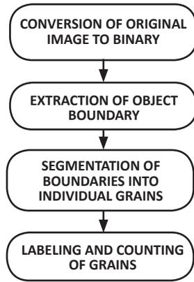
**Figure 5.** Algorithm for digital separation of touching grain images
