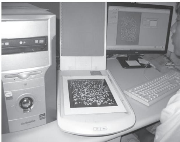
**Figure 6.** The prototype computer vision system consisting of a flatbed scanner (a) as the image acquisition device and a desktop computer (b)
