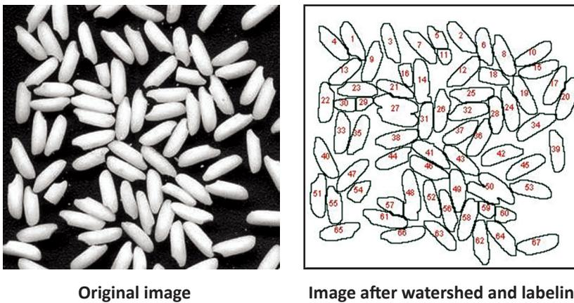
**Figure 11.** Image of medium grain milled rice before and after digital separation process showing some grains incorrectly separated
