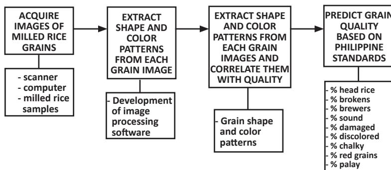
**Figure 1.** Conceptual framework for the proposed computer vision system for milled rice quality analysis
