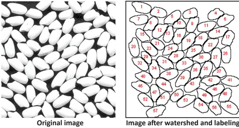
**Figure 10.** Image of short grain milled rice before and after digital separation process showing 100% separation.
